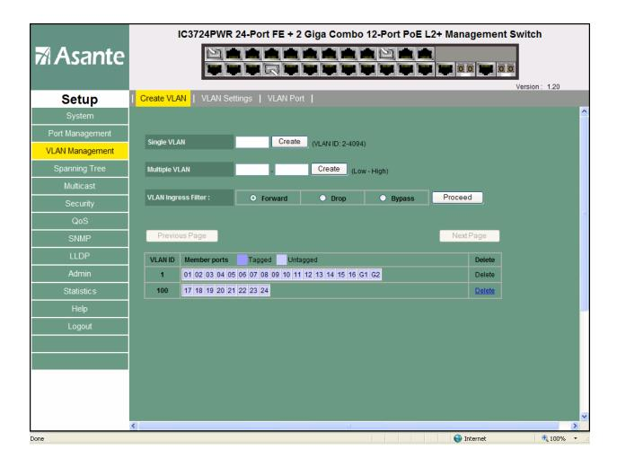
**VLAN MANAGEMENT – VLAN SETTINGS.** With a vlan selected, ports can be marked as tagged, or untagged. Lover on the screen, LAG groups can also be tagged or untagged. Click Save Settings when done.
